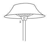
Step 10: Push the Heater Head onto the Top Tube and fix in position using the 2\*10mm screws.
