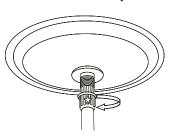
Step 6: Tighten the Plastic Fixation Part by screwing the Screw Knob.
