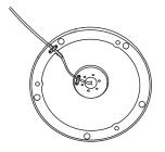
Step 11: Fix the Power Cord on the Iron Base by using 4\*15mmscrews.
